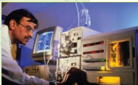
Figure 1.1.1 An instrumental analytical technique known as high performance liquid chromatography (HPLC) is used to test the purity of an experimental AIDS vaccine.
